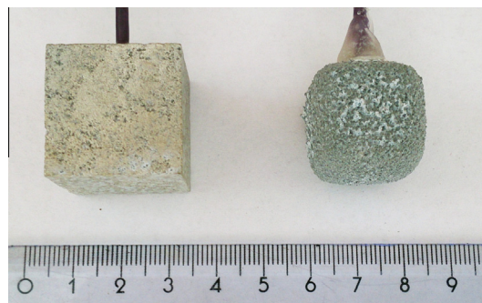
Fig. 6. Samples – anodes after the exposition. Transistor driven (left) and without the transistor driving system (right).
