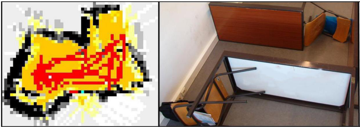
Fig. 4. Map (a) against reality (b) for LeJOS SLAM 9 .
