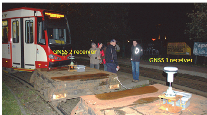
Fig. 1. Configuration of GPS/Glonass receivers on the platform
