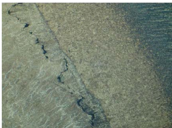
Fig. 5. Microstructure of the wet MMA welded joint made of S420G2+M steel; visible extensive crack on the boundary between the weld and HAZ. Mag. 50 \times .
