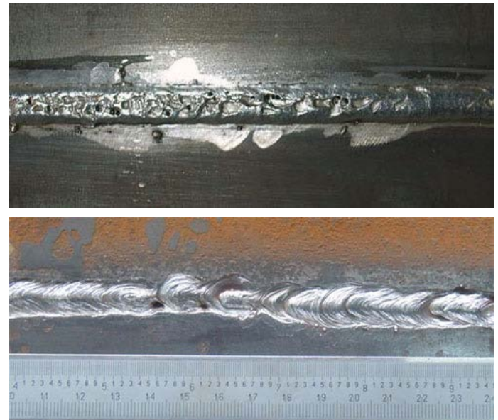
Fig. 2. Joints welded under water: a) S355J2G3 steel, flux-cored arc welding using the local dry chamber method, visible numerous gas pores; b) S420G2+M steel, wet MMA welding, visible undercuts and gas pores
