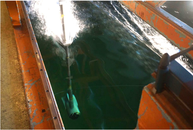
Fig. 10. View of the experimental underwater acoustic target mounted on the mobile platform while being measured at a speed equal to 4 m/s.
