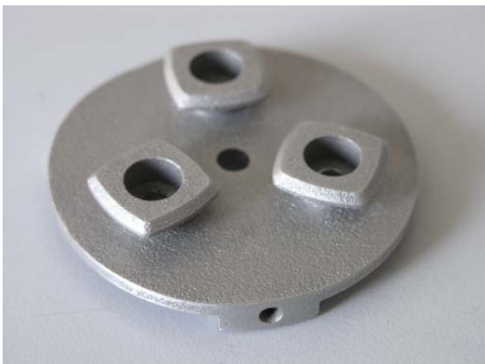
Fig. 7. Stator – contra-masse of the multicell piezoelectric motor
