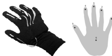
Fig. 1. eGlove device (left) and placement of the sensors (right)
