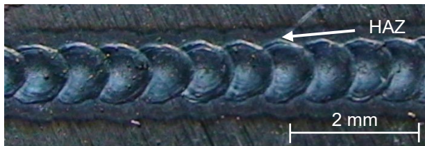
Fig. 2. Melted path produced by CO 2 laser beam and a luminescent plume formed on a sample of C80U steel in processing program 8, under 20× magnification, with a visible heat-affected zone (depicted by arrow).
