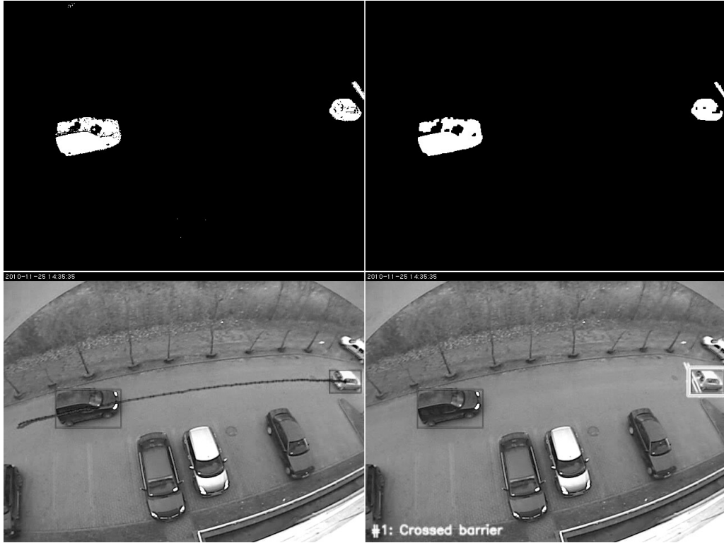
Figure 4: Example of video analysis results: background subtraction, morphological processing, object detection and tracking, event detection
