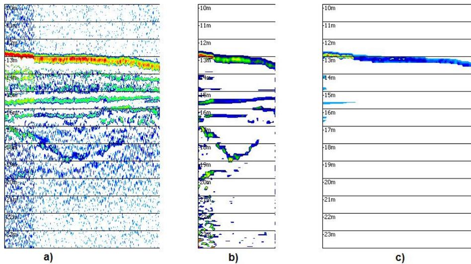
Fig. 3. Impact of the signal processing on the image of the same part of bottom (Gulf of Gdansk)
