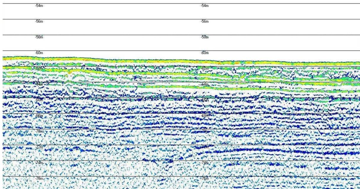
Fig. 6. Typical image obtained using the parametric echosounder
