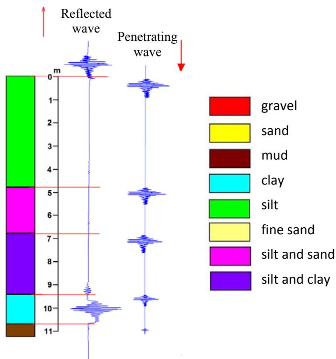
Fig. 5. Changes in shape of reflected and penetrating pulses during penetration of a bottom (an example of a core taken from the bottom of Gulf of Gdansk)
