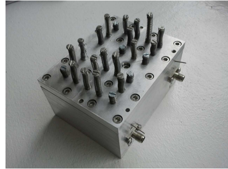
Fig. 13. Manufactured prototype of combline diplexer.
