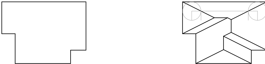
Figure 2: The Geometric Competition 2011: “Draw the construction of the roof. Assume that the planes which rise from the eaves parallel to the longest side have twice the slope of the other planes”
