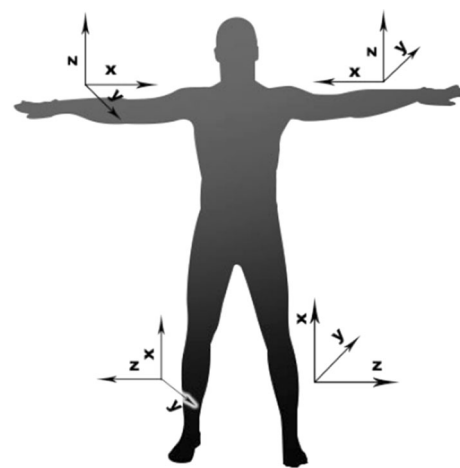
Fig. 1 Location of acceleration sensors on subject's body
