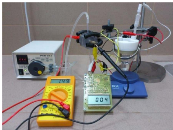
Figure 8. Enzymatic biobattery integrated with minipotentiostat and biosensor.
