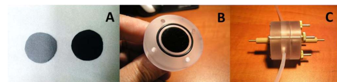
Figure 1. (A) Carbon Paper (CP) before and after modification, (B) Cathode contact in the biobattery (C) Construction of the biobattery designed for a flow system.
