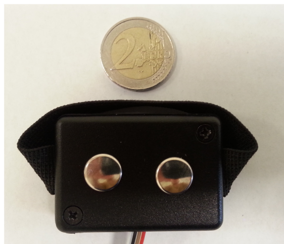
Fig. 5. Skin conductance sensor.
