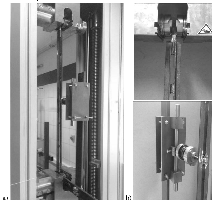
Fig. 7. Experimental set-up of the bar: a) front view of the structure placed at the strength testing machine Zwick Roell Z400, b) details at the supports
