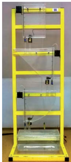
Rys. 1. Kaskada zbiorników Fig. 1. System of cascade tanks
