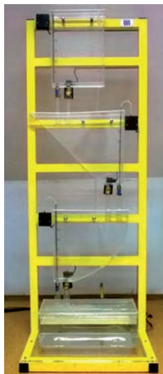
Rys. 1. Kaskada zbiorników Fig. 1. System of cascade tanks
