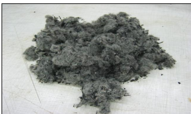
Fig. 1. Recycled textile fiber from used tires.
