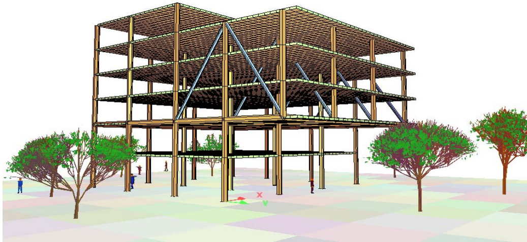
Fig.5. Numerical model of unique cantilever cablestayed structure.
