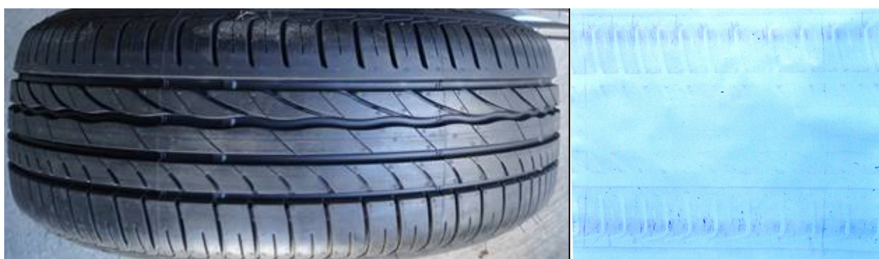
Fig. 13. Pressure distribution for RFT 205/55R16 tire tread section (tire without rubber insert) – visible increased pressure on the side sections of the tread, resulting from the reinforcement of tire sidewalls, which are in charge of transferring the forces during air-less driving (Fig. P. Stryjek ROSOMAK S.A.)
