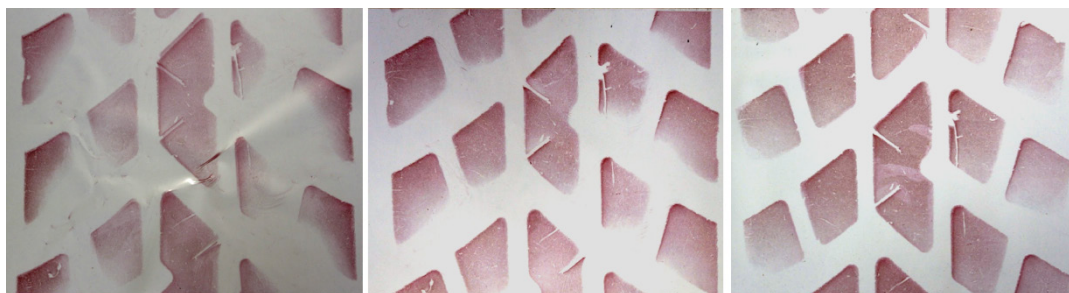
Fig. 12 Comparison of 14.00R20 tire treat marks in the KTO Rosomak transporter equipped with additional RunFlat insert (Fig. T. Nikisz ROSOMAK S.A.)
