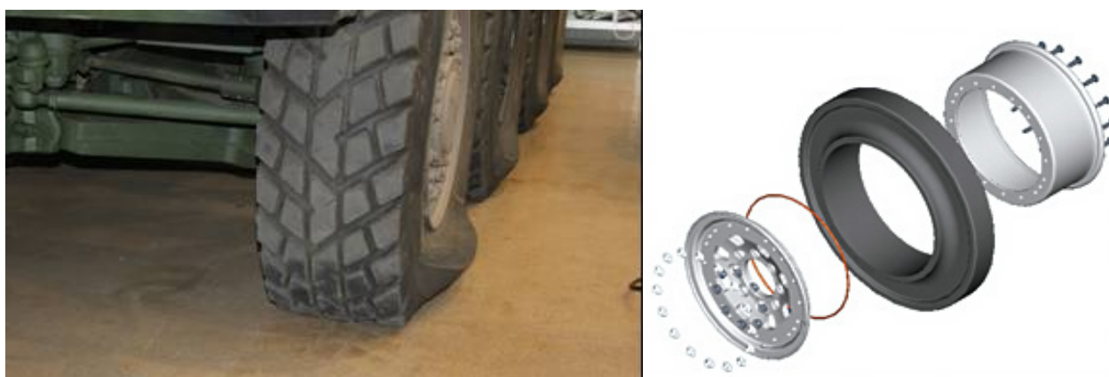
Fig. 4. On the left: view of a KTO Rosomak tire for 0 bar – with a RUN FLAT insert, on the right: a layout of the RUN FLAT system (Fig. T. Nikisz ROSOMAK S.A. / HUTCHINSON)
