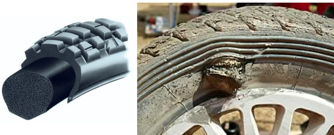
Fig. 7 View of the BIB MOUSSE system for motorcycle tires (permanent system) and a sports vehicle tire after damage and activation of the system (Fig. Michelin / www.automobilsport.com/race-categories-24,23584 )
