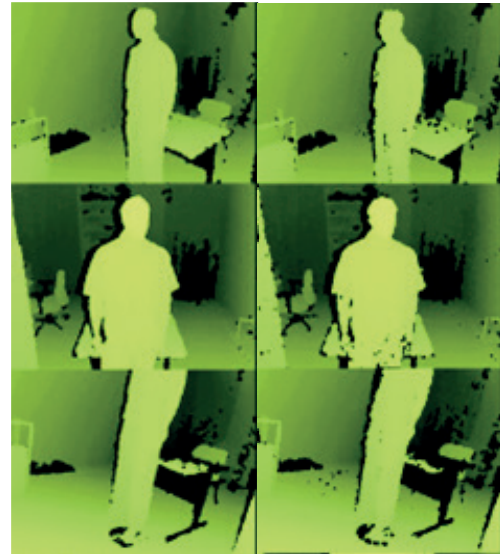
Fig 3. Effect of pre-processing using a vortex grid on a single frame (leaf= 0.01)
