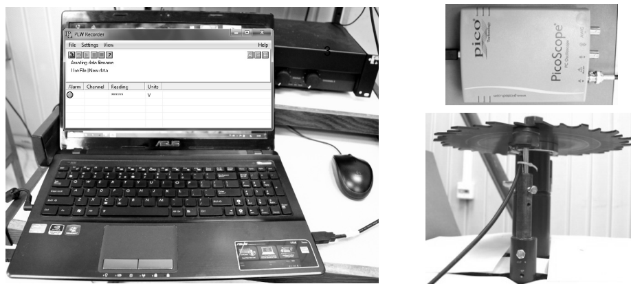
Fig. 3 Laboratory stand for testing circular saws with impact method, where: 1 – contactless inductive sensor, 2 – digital oscilloscope, 3 – NTB with software PicoLog Recorder
