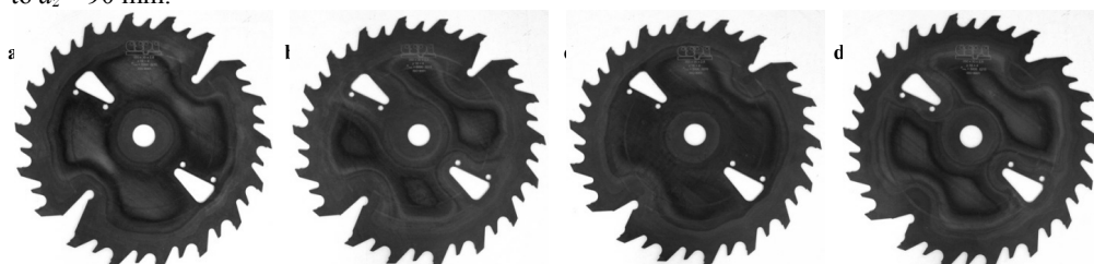
Fig. 1 Tested saw blades with external cut for cleaning knife with dimension equal to: a) 45 mm, b) 35 mm, c) 25 mm, d) 15 mm
