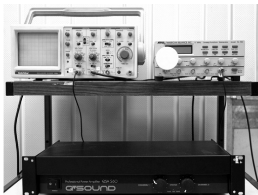
Fig. 2 Laboratory stand for testing circular saws with harmonic method, where: 1 – input function generator, 2 – signal amplifier, 3 – oscilloscope, 4 – inductor, 5 – contactless magneto-inductive sensor
