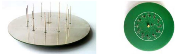
Fig. 3. Realized ESPAR antenna (top and bottom).
