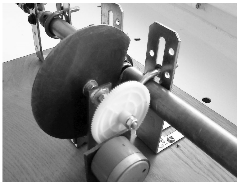
Fig. 7. Details of choking throttle
