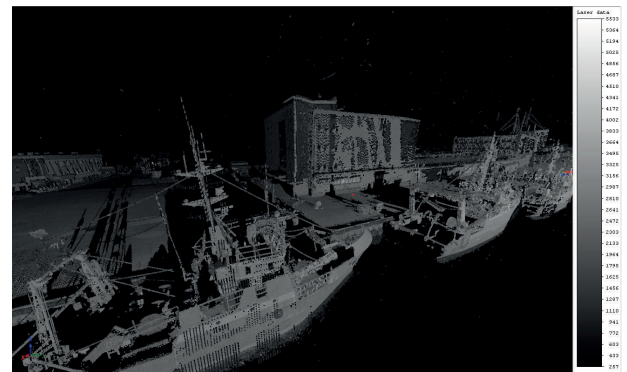
Fig. 12. MarLS visualization for vessels in harbour and port infrastructure (Laser data – number of points per square meter)
