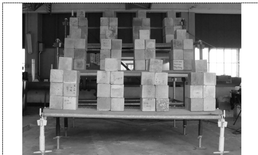
Figure 4. Front view of occupied steel temporary grandstand.
