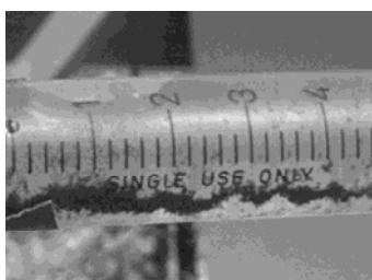
Fig. 7. Test tube with ferromagnetic dust in water (before shaking)
