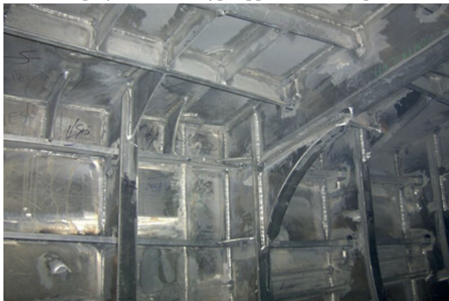
Fig. 1. Typical T-joints in ship structure
