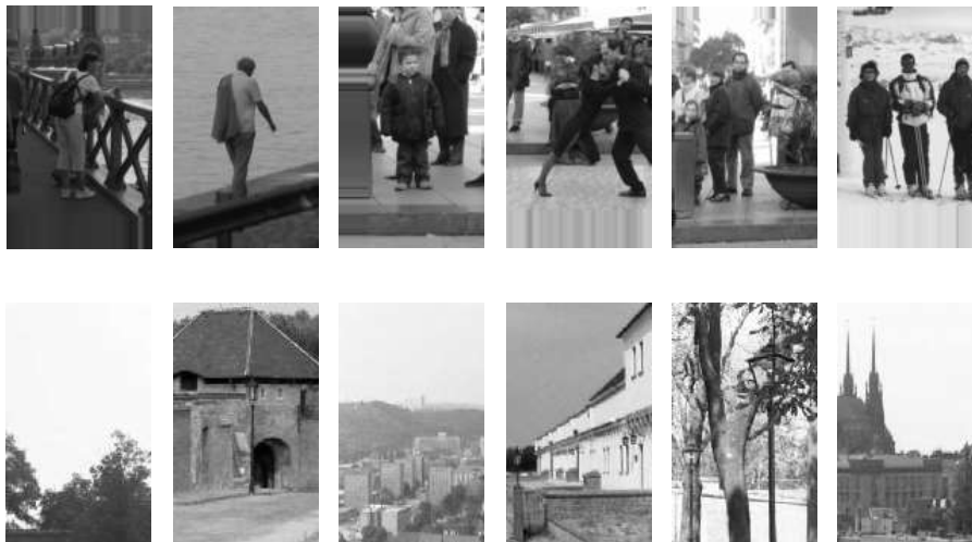
Fig 3 Few examples of positive images containing pedestrians (top row) and negative, nonpedestrian images (bottom row) from INRIA database [21].
