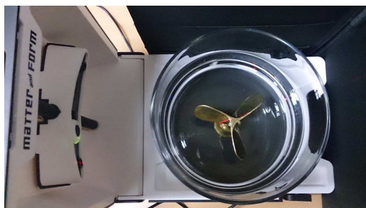
Fig. 7. Measurement in a round vessel in a series of measurements without water [own research].
