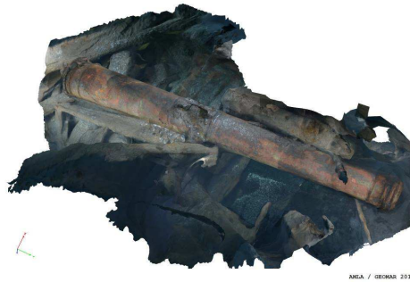
Fig. 16 A fragment of a point cloud generated from underwater photographs [10].
