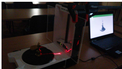
Fig. 6. Measurement through a sheet of plexiglass [own research].
