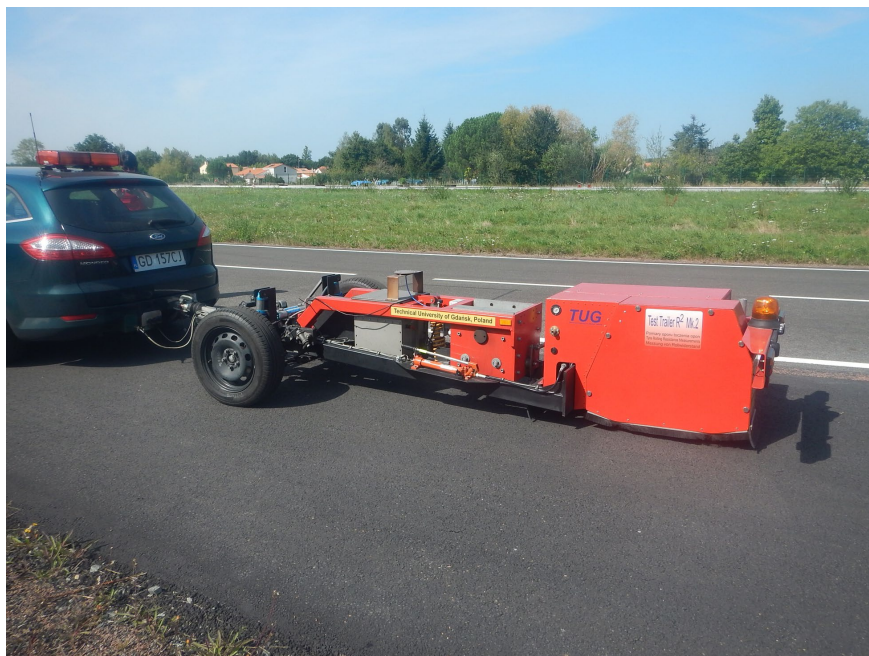
Figure 9. Rolling resistance test trailer R^2 Mk.2
