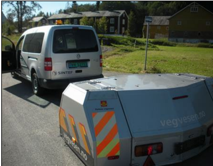
Figure 9. CPX test trailer used by SINTEF, Norway
