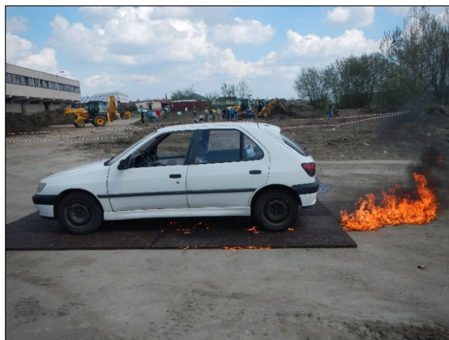
Figure 12. Car fire 30 s after ignition. Observe the fuel spill at right side of a car that is still not ignited [12].
