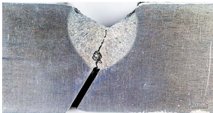
Fig. 5. Cross-section of the joint welded under water: specimen W4, non-saline water, q_{el} = 3.02 kJ/mm; the crack visible in the weld (initiated in the root); gas pore; etchant: Beraha
