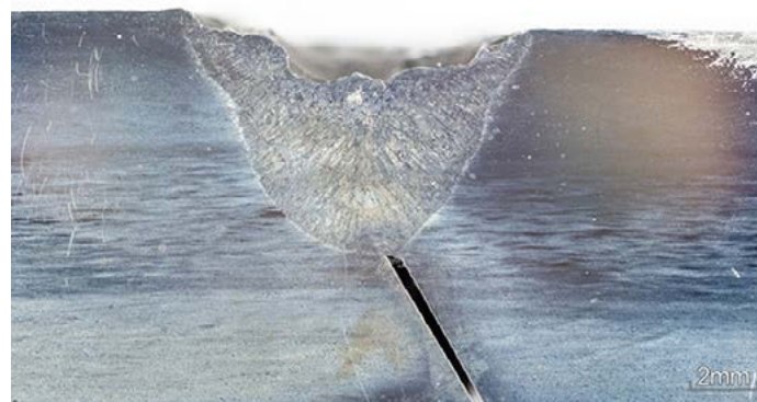
Fig. 4. Cross-section of the joint welded under water: specimen W3, non-saline water, q_{el} = 3.02 kJ/mm; the lack of welding imperfections; etchant: Beraha
