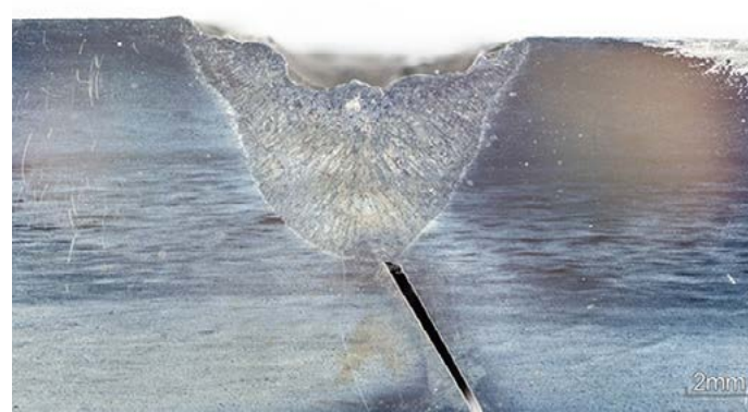
Fig. 4. Cross-section of the joint welded under water: specimen W3, non-saline water, q_{el} = 3.02 kJ/mm; the lack of welding imperfections; etchant: Beraha
