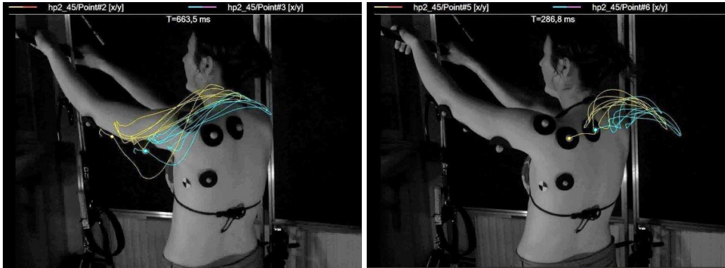
Fig. 7. Repetitiveness of the movement trajectory obtained under laboratory conditions
