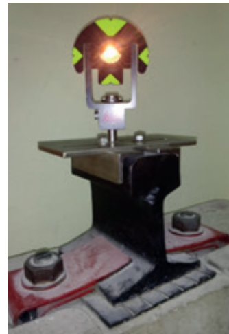
Fig. 1. Clamp with central point and mini prism Source: photo from own collection
