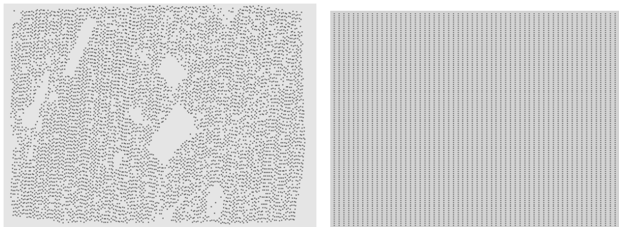
Fig. 3 Decreased TSset a) by means of reduction – Rset (source: own study in own software), b) by conducting GRID generation - Gset (source: own study in Surfer v.8).
