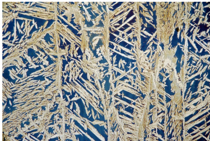
Fig. 7. Weld metal microstructure (W1). Magn. 100x
