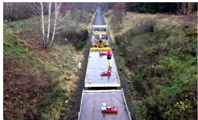
Figure 1: Configuration of GNSS receivers on the PWM-15 platforms.
