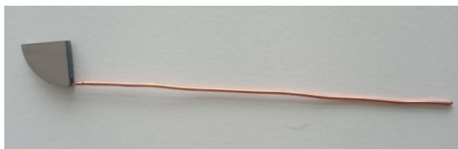
Fig. 3. The Ti13Zr13Nb alloy sample
