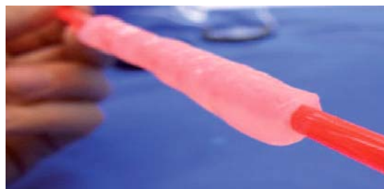
Fig. 8. Tube, acting as a blood vessel, made of BNC presented on a red glass, symbolizing the blood flow [49]
