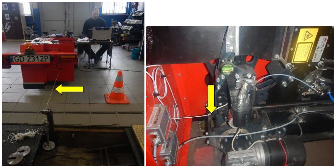
Figure 12. Calibration of R 2 Mk.2 trailer - force calibration (arrows indicate flexible rope pulling the test wheel spindle).
