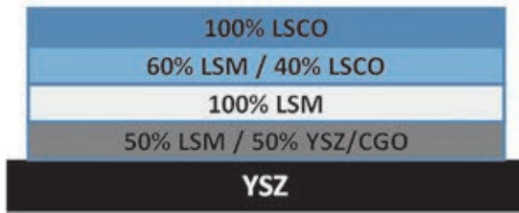
Fig. 1. Diagram of half-cell with gradient cathode on YSZ substrate [25]
