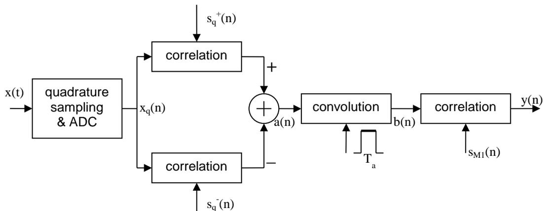
Fig. 8. Functional diagram of the receiver.
