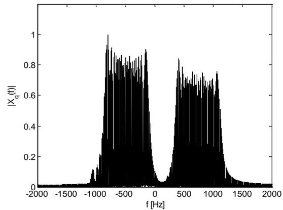
Fig. 7. Amplitude spectrum of echo signal ( $v = 10$  m/s).
