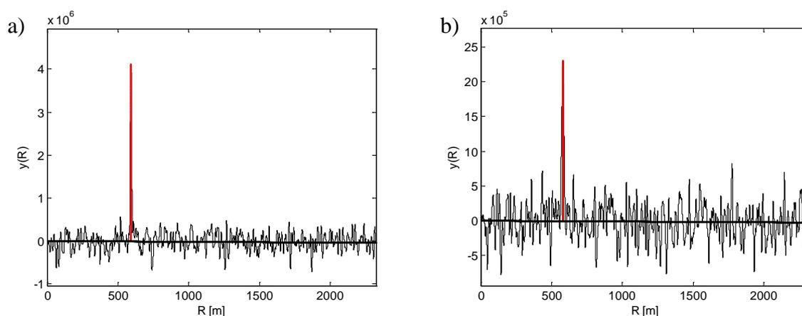
Fig. 17. The effect of target speed on output signal parameters for  $\text{SNR}_i = 0$  dB:
