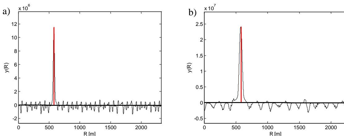
Fig. 15. The effect of selecting the order  $N$  of MLS sequences and duration  $T_e$ : a)  $N = 5$ ,  $T_e = 0.1$  s, b)  $N = 4$ ,  $T_e = 0.2$  s. ( $f_0 = 10$  kHz,  $B = 2$  kHz,  $B_e = 0.4$  kHz,  $p = 0.2$ ,  $v = 5$  m/s).
