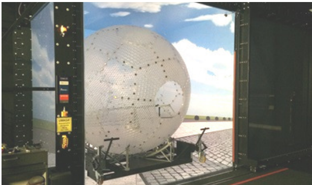
Fig. 2 The spherical walk simulator inside the CAVE in the I3DVL (the gate of the CAVE is open)
