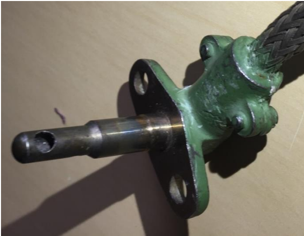
Img 7. Gas stream temperature measuring thermocouples a) single-point with a covered junction b) four-point with a covered junction
