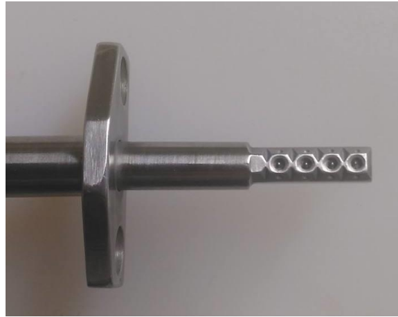
Img 7. Gas stream temperature measuring thermocouples a) single-point with a covered junction b) four-point with a covered junction
