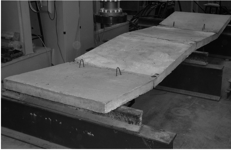
Fig. 8. Mode of failure slabs C-1 and C-2
