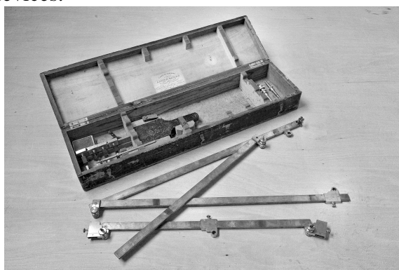
Illustration 1: Collection of Prof. H. Limon: Pantograph, company Adrien Cavard, Paris – photo K. Krzempek
