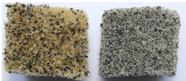
Fig. 3. Rigid PU foams modified with untreated (left) and thermomechanically reclaimed GTR (right) [71]
