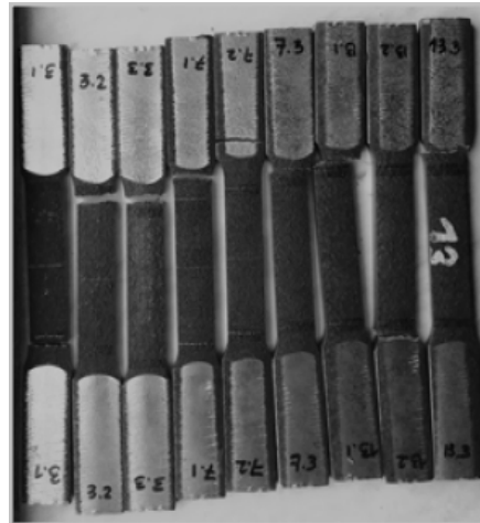
Fig. 7. Specimens with rectangular cross-section of 25x10 mm after tests
